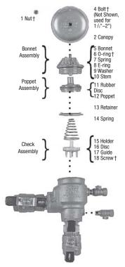
Illustration shown is for sizes  $\frac{3}{4}$ " through  $\frac{1}{4}$ " only. Bonnet and bolt for  $\frac{1}{2}$ " and  $\frac{2}{4}$ " not shown.
